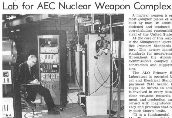
ROSS BIRDSALL of Nuclear Standards Section 2411-3 is performing preliminary measurements in the Cockcroft-Walton Accelerator target area in preparation for calibration of high energy neutron detectors. One of the detectors, a silver activation detector, is mounted on stand at right of accelerator target tube.
